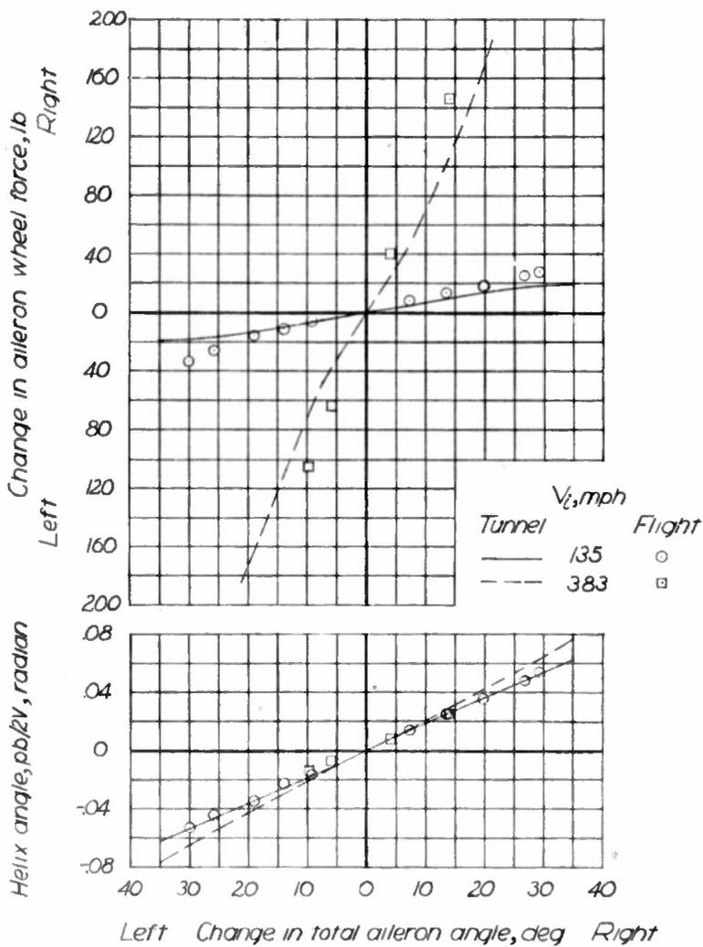
Figure 16. - Variation of aileron wheel force and helix angle  $pb/2V$  with change in total aileron angle in rolls with rudder fixed, flaps retracted, and rated power.
