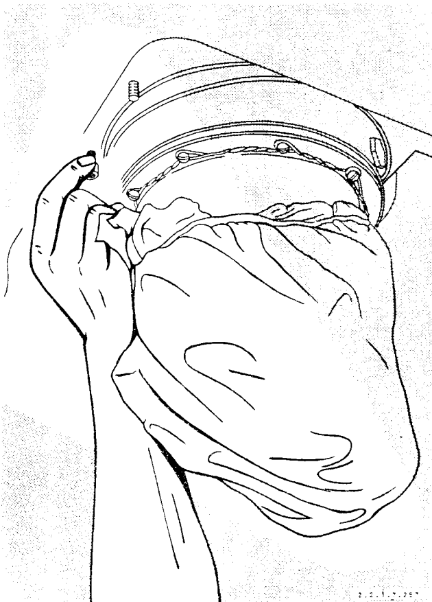
Figure 2-15. Installing Sighting Station Lower Attaching Bolts
