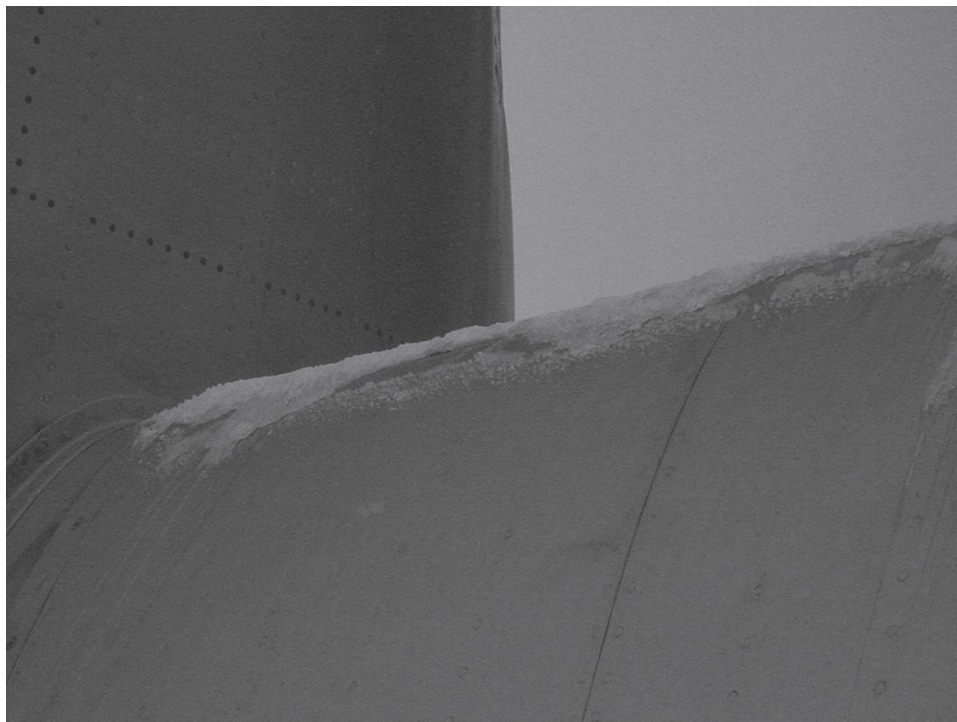
FIG. 11. A photograph of glaze ice on the Convair taken after experiencing aircraft icing between 2152 and 2207 UTC.
