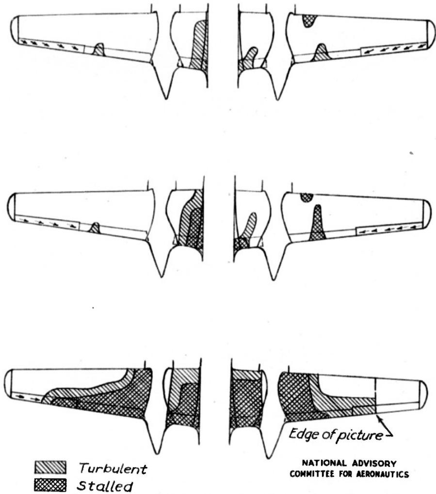
Figure 8.- Diagrams of stall progression in the gliding condition. Engines idling; flaps and landing gear up; cowl flaps closed; oil cooler one-half open; Douglas A-26B airplane.
