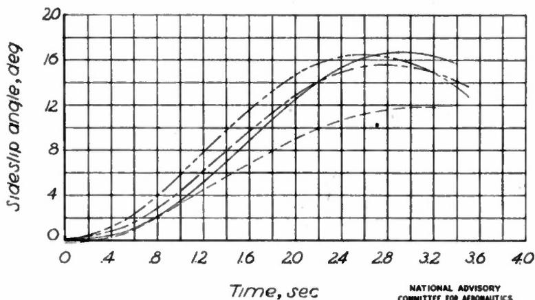
Figure 17.- Rolling velocity and sideslip during aileron roll out of  $30^\circ$  banked turn.  $\delta_r = 0^\circ$ ;  $V_i = 145$  miles per hour at 10,000-foot altitude; level flight power.
