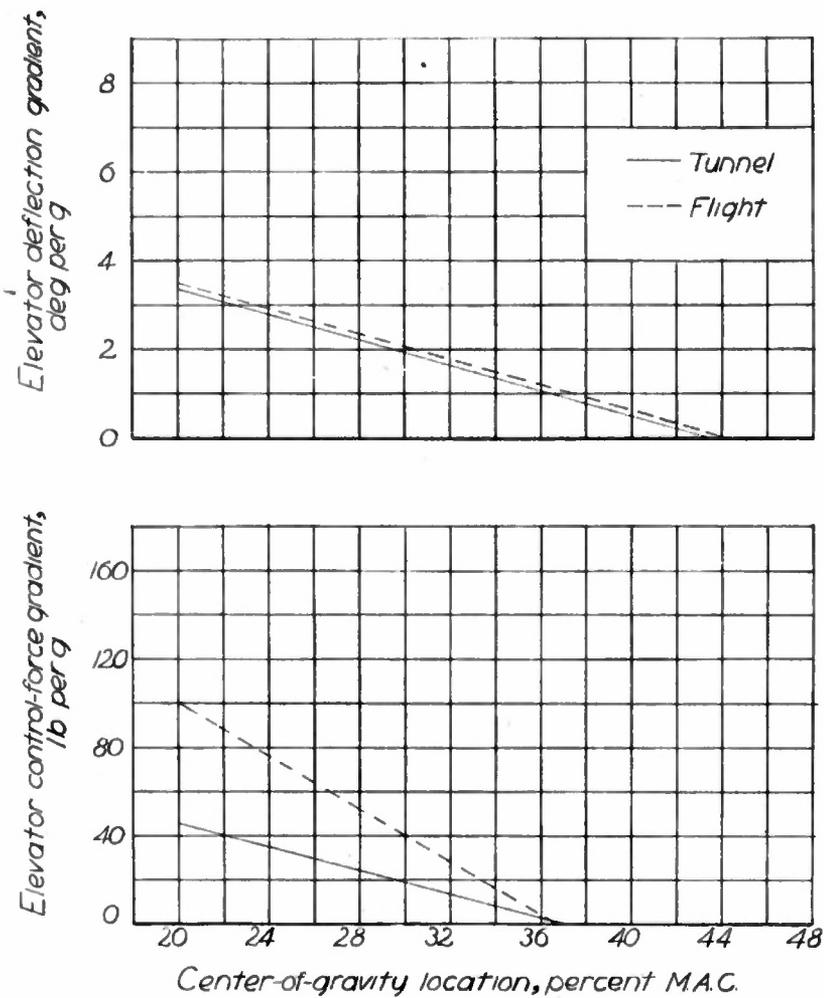
Figure 7.-Variation of elevator control-force and deflection gradients with center-of-gravity location.  $V_i=260$  miles per hour at 10,000-foot altitude;  $\delta_f=0^\circ$ ; rated power; steady turning flight.
