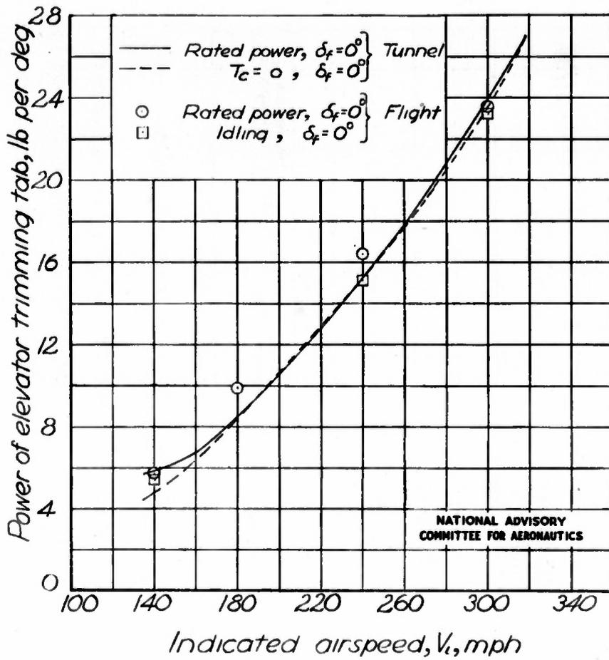
Figure 4.-Variation of elevator trim-tab effectiveness with airspeed.
