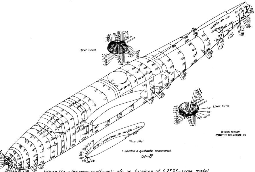
Figure 17a.— Pressure coefficients p/q on fuselage of 0.2375-scale model
