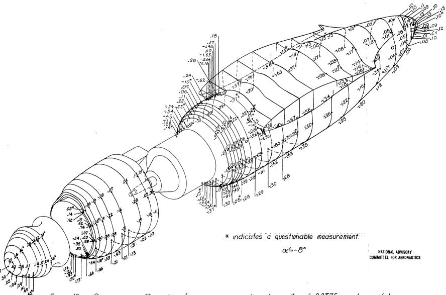
Figure 12 a.—Pressure coefficients p/q on spinner, cowl, and nacelle of 0.2375-scale model Douglas XA-26 airplane;  $\psi=5^\circ$ ;  $q\approx50$ lb/sqft;  $R\approx3,870,000$ ;  $M\approx0.12^\circ$ .
