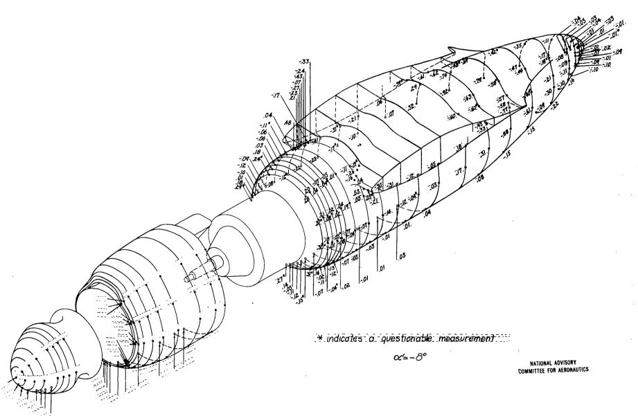
Figure 14a.—Pressure coefficients p/q on nacelle of 0.2375-scale model Douglas XA-26 airplane;  $\psi=0^\circ; \delta_f=55^\circ; q\approx 50\,lb/sqft; R\approx 3,720,000; M\approx 0.12$ .
