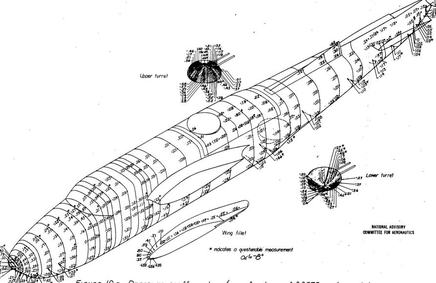
Figure 19 a - Pressure coefficients p/q on fuselage of 0.2375-scale model Douglas XA-26 airplane; \psi=10°; q \sigmu 50 lb/sqft; R \sigmu 3,950,000; M \sigmu 0.12.
