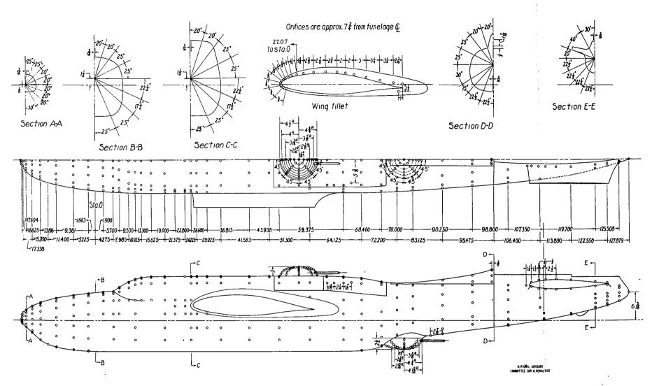
Figure 4.-Location of orifices on fuselage of 0.2375-scale model of Douglas XA-26 airplane
