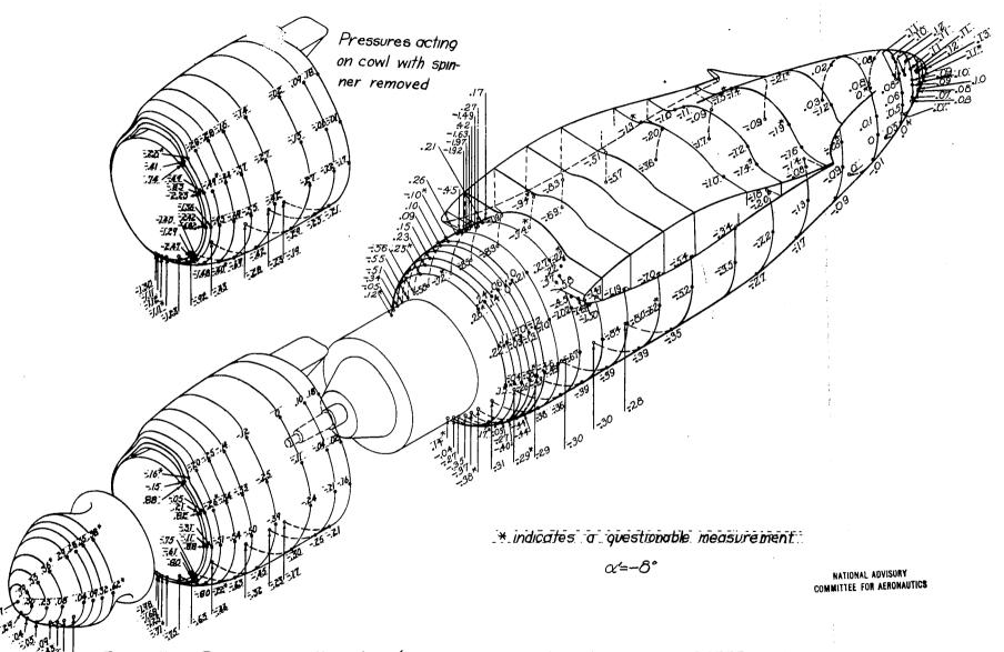
Figure II a.—Pressure coefficients p/q on spinner, cowl, and nacelle of 0.2375-scale model Douglas XA-26 airplane;  $\psi=0^\circ$ . Test conditions with spinner installed;  $q\approx50$ lb/sqft;  $R\approx3,880,000$ ;  $M\approx0.12$ . Test conditions with spinner removed;  $q\approx35$ lb/sqft;  $R\approx3,300,000$ ;  $M\approx0.10$ .
