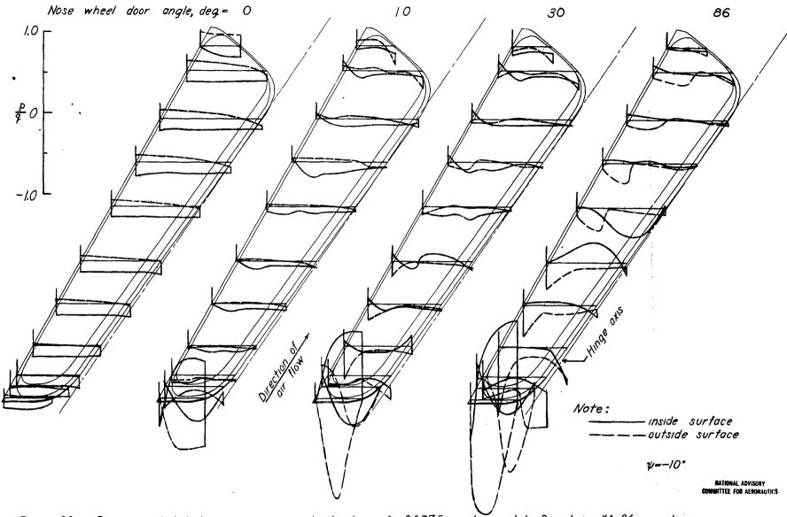
Figure 22 a.—Pressure distribution over nose wheel door of 0.2375-scale model Douglas XA-26 airplane; \alpha=4°; q=50 lb/sq ft; R =3,940,000; M = 0.12.
