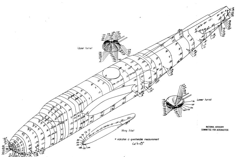
Figure 18 a. — Pressure coefficients p/q on fuselage of 0.2375-scale model Douglas XA-26 airplane;  $\psi=5^\circ$ ;  $q\approx50$ lb/sqft;  $R\approx3$ ,970,000;  $M\approx0.12$ .
