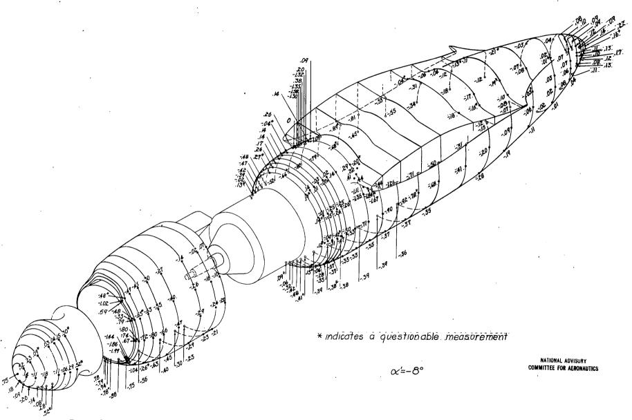
Figure 9a.—Pressure coefficients p/q on spinner, cowl, and nacelle of 0.2375—scale model Douglas XA-26 airplane;  $\psi=-10^\circ$ ;  $q\approx 50$  lb/sq ft;  $R\approx 3$ ,900,000;  $M\approx 0.12$ .
