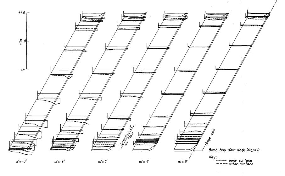
Figure 23a .— Pressure distribution over bomb bay door of 0.2375-scale model Douglas XA-26 Airplane;  $\psi=0^\circ; q\approx 50$ lb/sq ft;  $R\approx 3,640000; M\approx 0.18$ .
