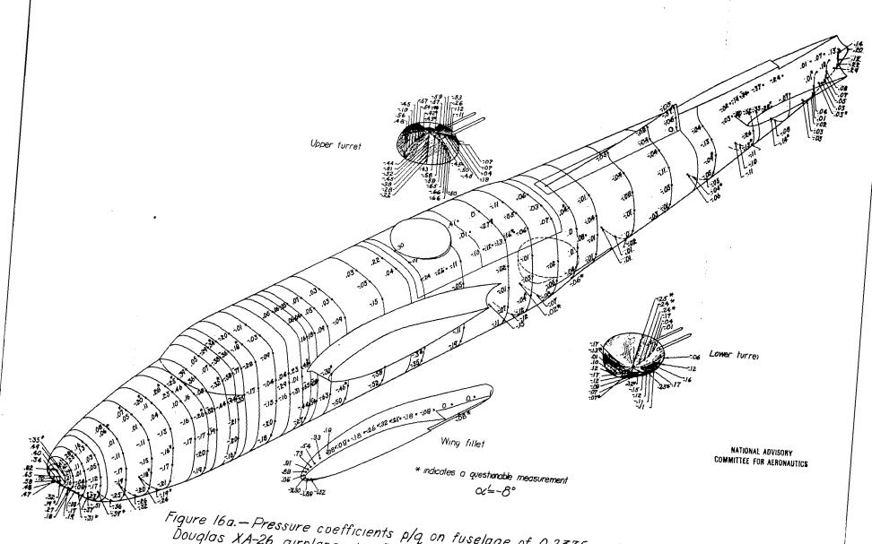
Figure 16a.—Pressure coefficients p/q on fuselage of 0.2375-scale model Douglas XA-26 airplane;  $\psi=-5^\circ$ ;  $q\approx50$  lb/sq ft;  $R\approx3$ ,990,000;  $M\approx0.12$ .
