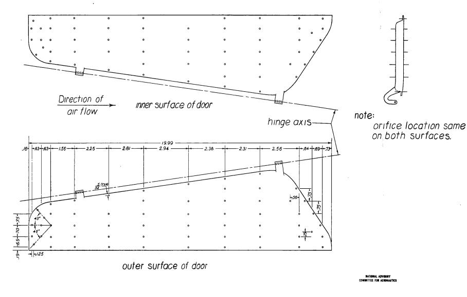
Figure 6-Location of orifices on nose wheel door of 0.2375-scale model Douglas XA-26 airplane
