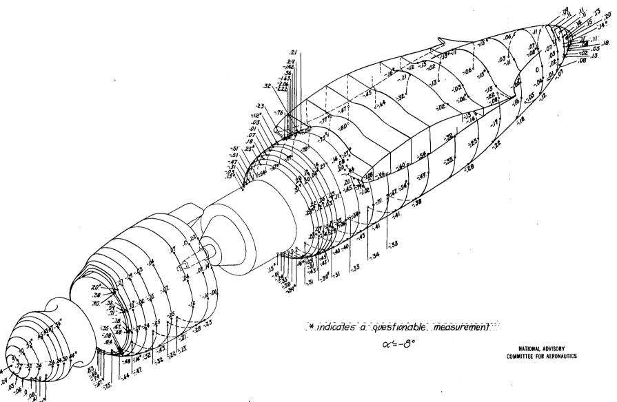
Figure 13 a. — Pressure coefficients p/q on spinner, cowl, and nacelle of 0.2375—scale model Douglas XA-26 airplane;  $\psi$ =10°;  $q\approx$ 501b/sqft; R $\approx$ 3,870,000; M $\approx$ 0.12.
