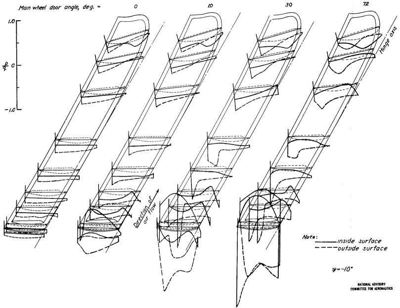
Figure 21a.—Pressure distribution over main wheel door of 0.2375-scale model Douglas XA-26 airplane;  $\alpha = 4$ ;  $q \approx 50$  lb/sq ft;  $R \approx 3,950,000$ ;  $M \approx 0.12$ .
